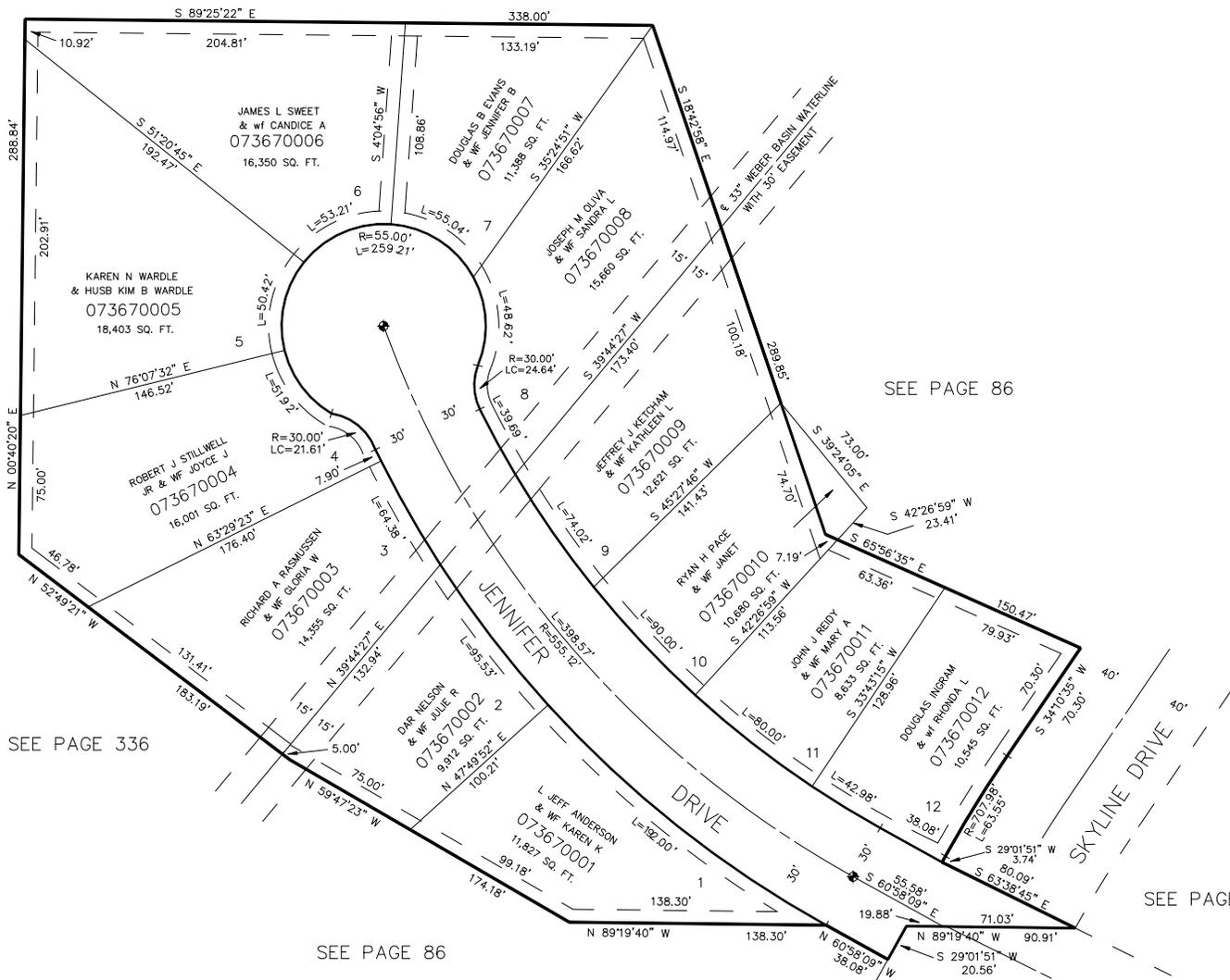
7' UTILITY & DRAINAGE EASEMENTS EACH SIDE OF PROPERTY LINES AS INDICATED BY DASHED LINES EXCEPT AS OTHERWISE SHOWN.
